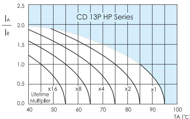
$I_a$  = actual ripple current at 120Hz,  $I_r$  = rated ripple current at 120Hz, 85°C
