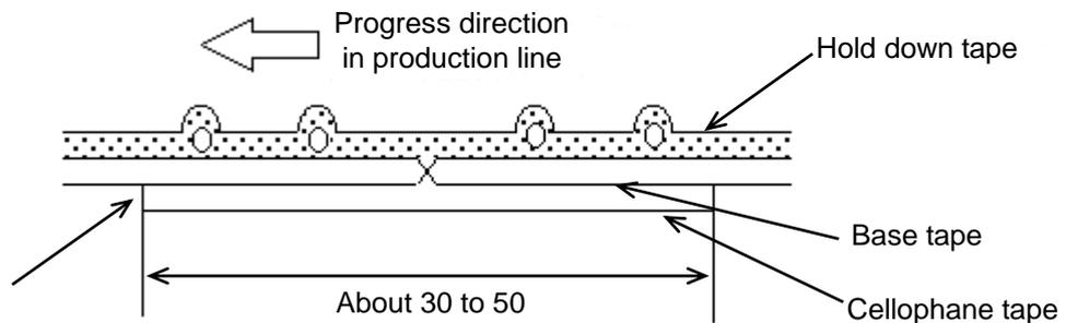
No lifting for the direction of progressing
