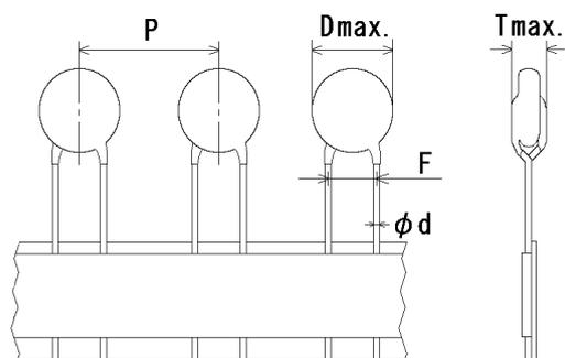
Note) The mark '\*' of lead code differ from lead spacing(F), lead diameter(d) and pitch of component(P). Please see the following list or taping specification about details.
