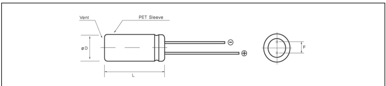
**Note : It is not allowed to go through reflow (IR, Atmosphere heating methods etc.) process**
