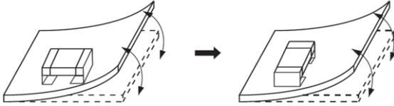
Locate chip horizontal to the direction in which stress acts.
