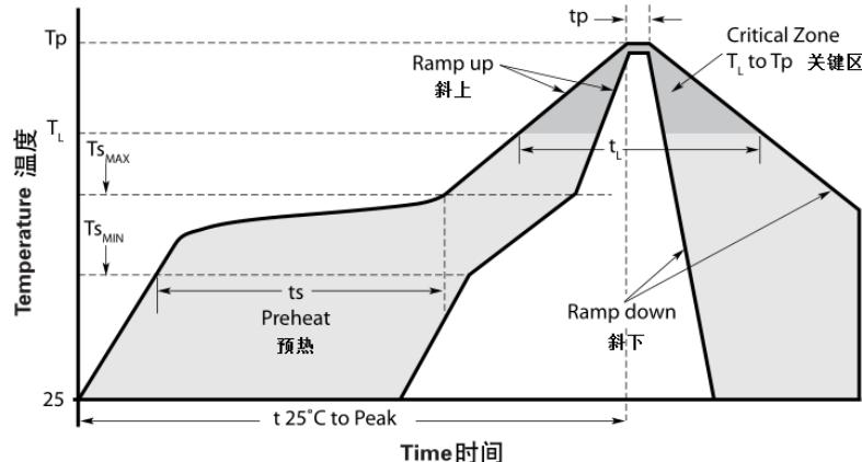
Recommended reflow methods: IR, hot air oven, N2 environment for lead-free. 推荐回流焊方法：红外线，热空气，氮气，无铅。
