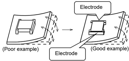
(2) Components location on PCB separation
