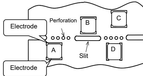
(3) Mounting components near screw holes
