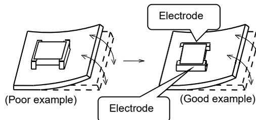
(2) Components location on PCB separation
