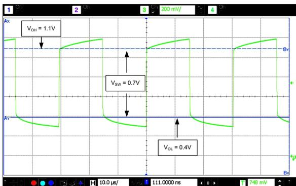
Figure 4. SiT1533AI-H4-D14-32.768 Output Waveform (10 pF load)
