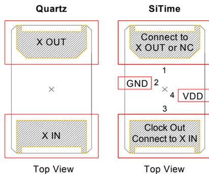
**Figure 2. SiT1533 Footprint Compatibility with Quartz XTAL Footprint [6]**
