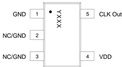
**Figure 1. Pin Assignments**
