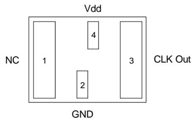
**Figure 2. Pin Assignments**
