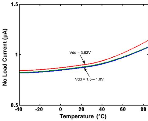
Figure 7. Supply Current Over Temperature (No Load)
