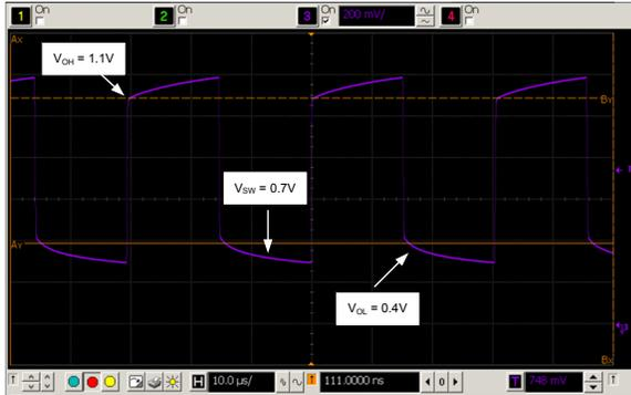
**Figure 2. SiT1552AI-J4-D14-32.768 Output Waveform (10 pF load)**
