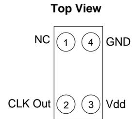
Figure 1. Pin Assignment
