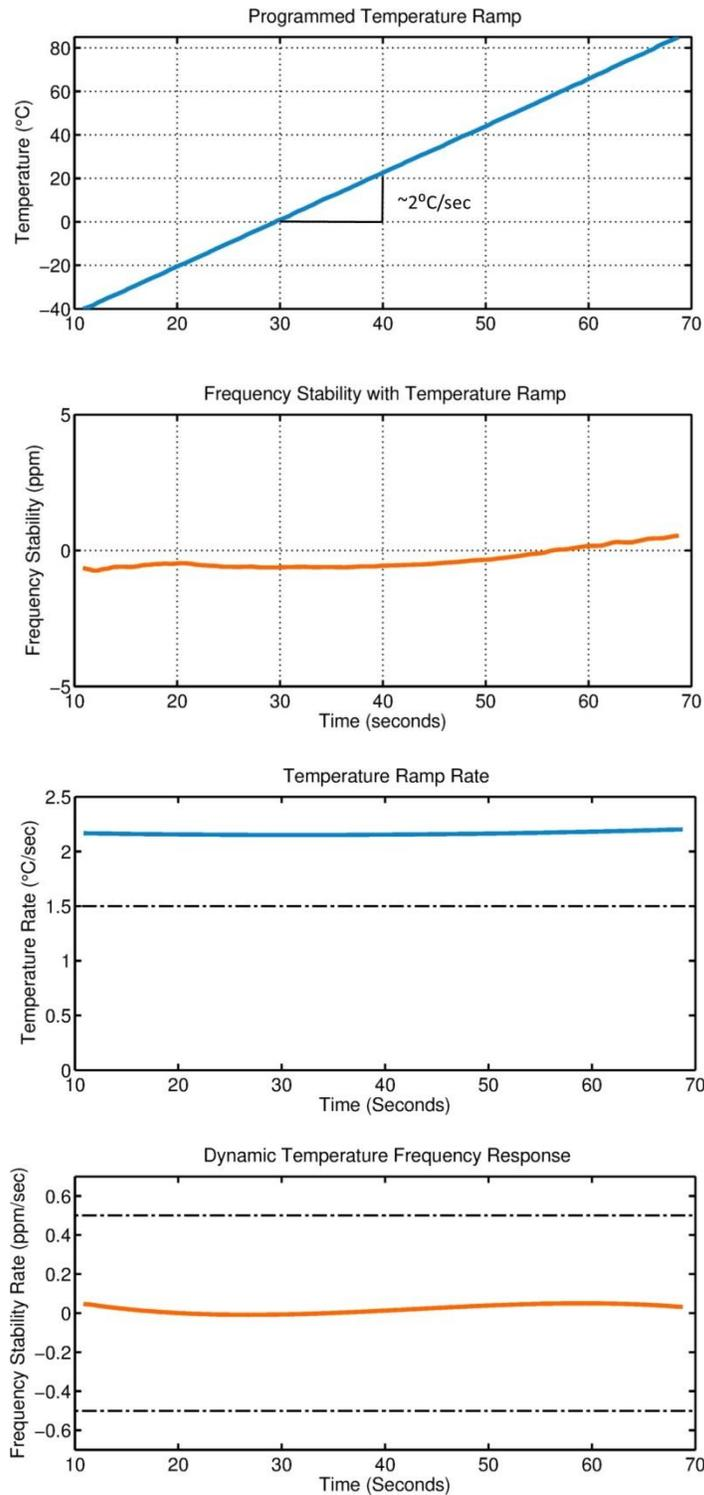
Frequency accuracy under a moderate temperature ramp up to  $2^{\circ}\text{C}/\text{sec}$  is limited by the TCXO's trimmed accuracy of the frequency stability over-temperature.
