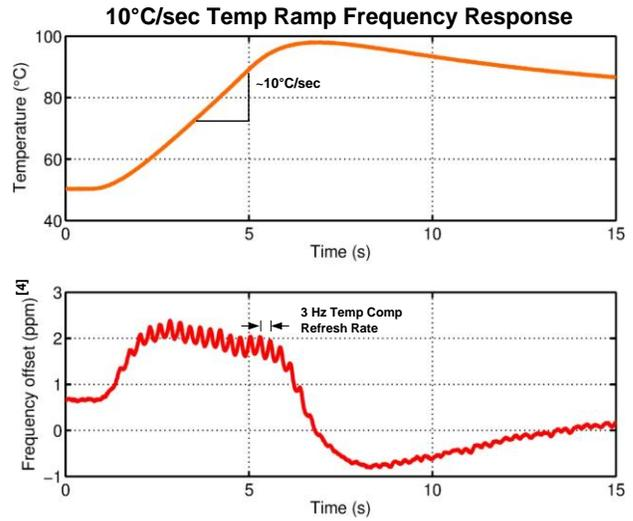
For temperature ramps  $>5^{\circ}\text{C}/\text{sec}$ , the frequency accuracy is limited by the update rate of the temperature compensation path (see the  $5^{\circ}\text{C}/\text{sec}$  and  $10^{\circ}\text{C}/\text{sec}$  plots).
