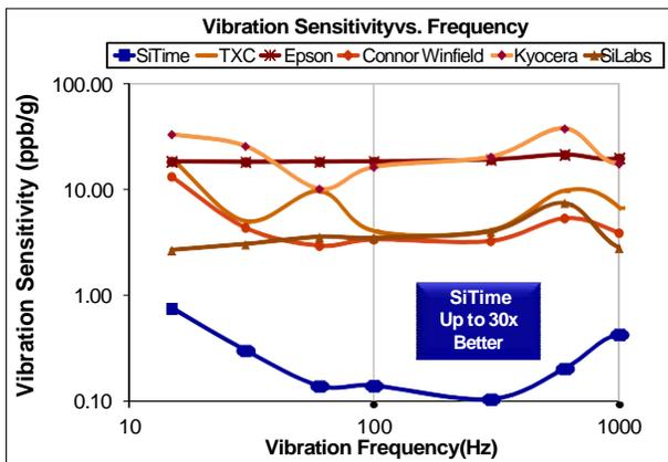
Figure 5. Vibration Robustness<sup>[5]</sup>
