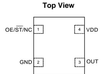
**Figure 1. Pin Assignments**
