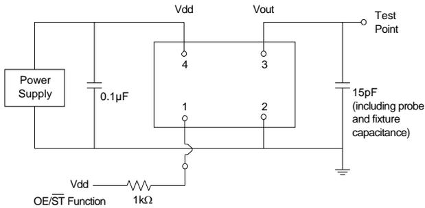
**Figure 2. Test Circuit**
