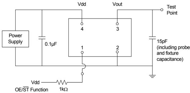
**Figure 2. Test Circuit**
