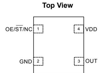
**Figure 1. Pin Assignments**
