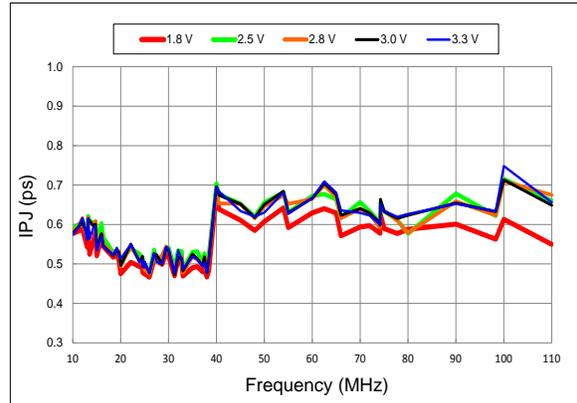
Figure 14. RMS Integrated Phase Jitter Random (900 kHz to 20 MHz) vs Frequency<sup>[9]</sup>
