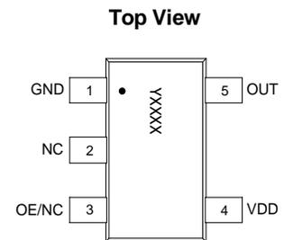
Figure 1. Pin Assignments
