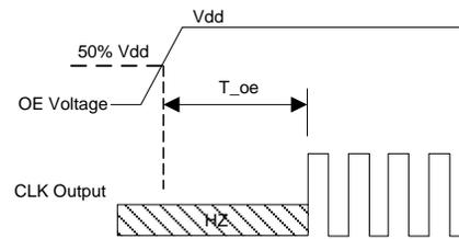
T\_oe: Time to re-enable the clock output
