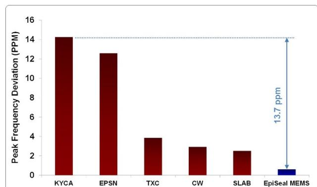
Figure 4. Power Supply Noise Rejection<sup>[4]</sup>
