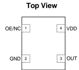
**Figure 1. Pin Assignments**
