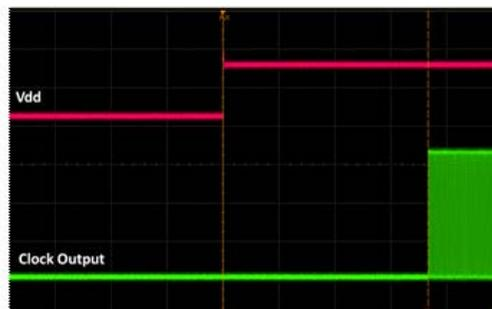
**Figure 16. Startup Waveform vs. Vdd**
