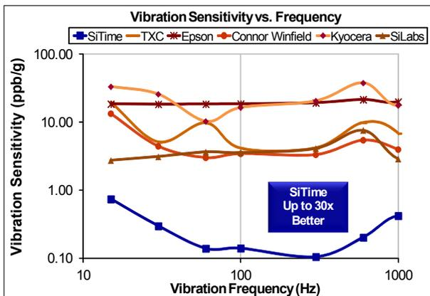
Figure 5. Vibration Robustness<sup>[5]</sup>
