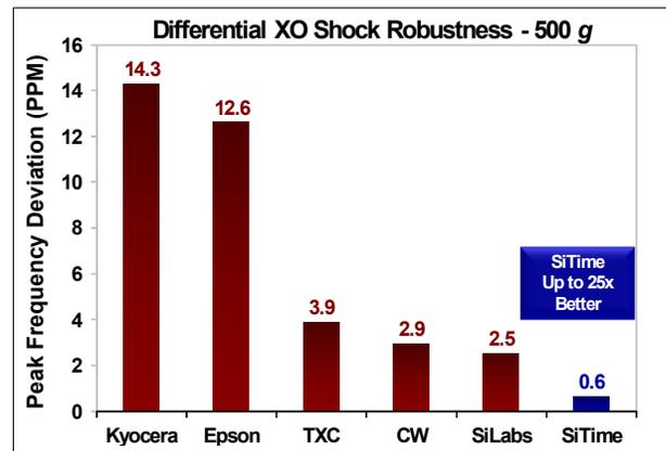
Figure 6. Shock Robustness<sup>[6]</sup>
