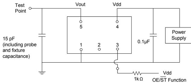
**Figure 2. Test Circuit**
