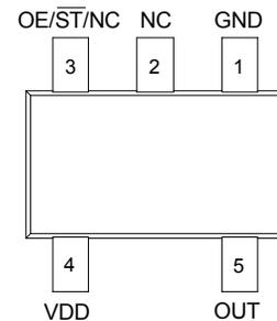
Figure 1. Pin Assignments
