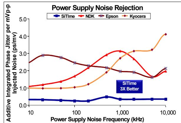
Figure 4. Power Supply Noise Rejection<sup>[4]</sup>
