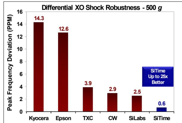
Figure 6. Shock Robustness<sup>[6]</sup>
