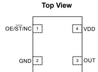
**Figure 1. Pin Assignments**
