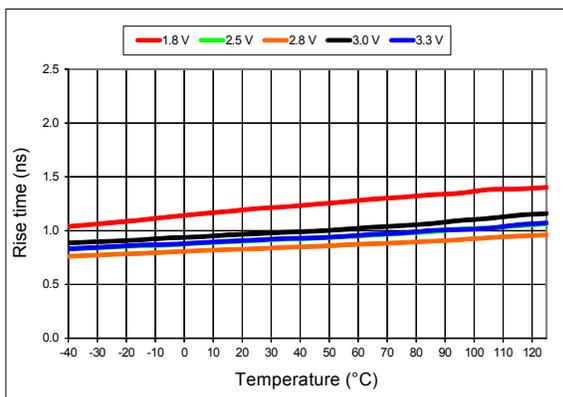
Figure 12. 20%-80% Rise Time vs Temperature (125 MHz Output)
