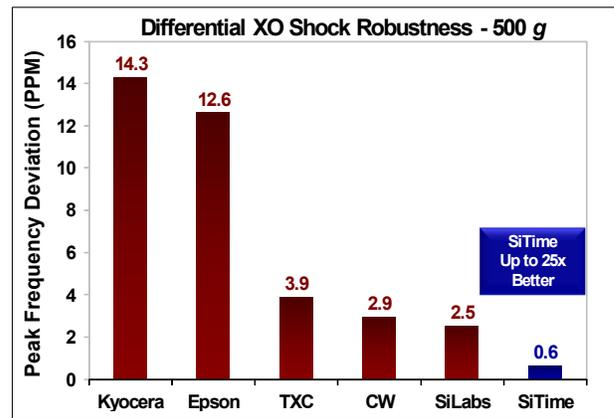
Figure 6. Shock Robustness<sup>[6]</sup>
