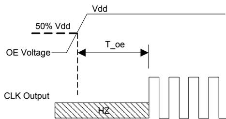
$T_{oe}$ : Time to re-enable the clock output
