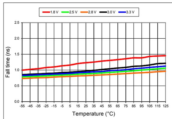
Figure 13. 20%-80% Fall Time vs Temperature (125 MHz Output)
