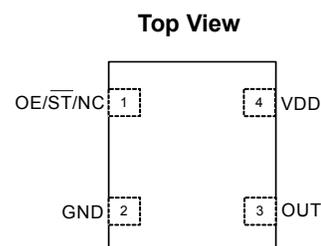
**Figure 1. Pin Assignments**
