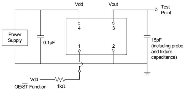
**Figure 2. Test Circuit**
