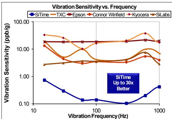
Figure 5. Vibration Robustness<sup>[5]</sup>
