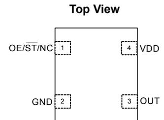
**Figure 1. Pin Assignments**
