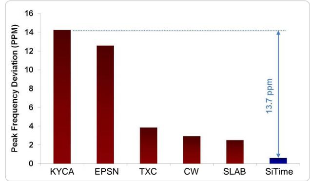
Figure 6. Shock Robustness<sup>[6]</sup>
