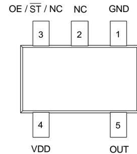
Figure 1. Pin Assignments
