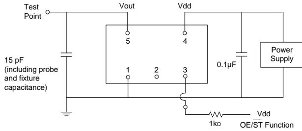
Figure 2. Test Circuit
