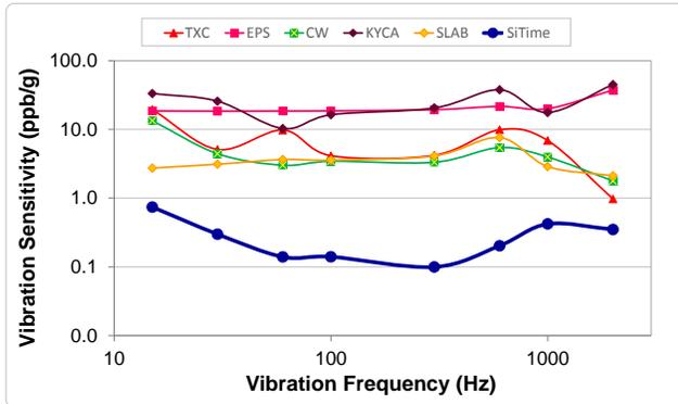
Figure 5. Vibration Robustness<sup>[5]</sup>
