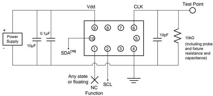
**Figure 13. Clipped Sinewave Test Circuit (I<sup>2</sup>C Control), DCTCXO mode for AC and DC Measurements**
