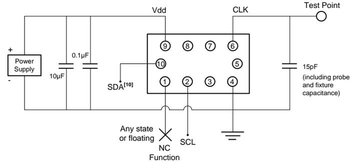
**Figure 12. LVCMOS Test Circuit (I<sup>2</sup>C Control), DCTCXO mode**
