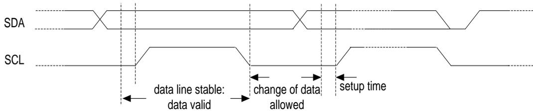
**Figure 43. Data and clock timing relation in I<sup>2</sup>C bus**
