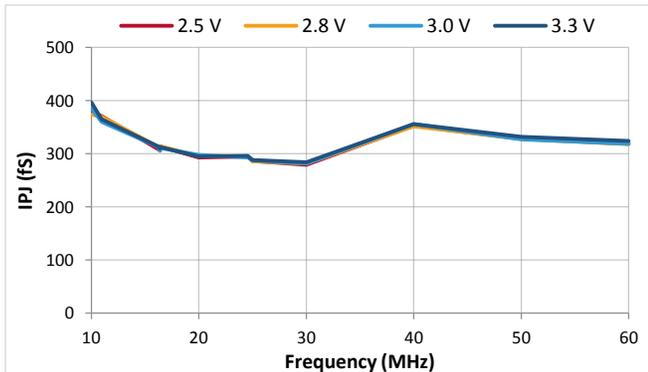
Figure 33. T<sub>phj</sub>, RMS Random, VTCXO (Clipped Sine)
