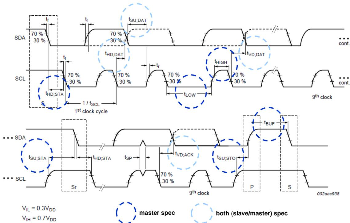
Figure 48. I<sup>2</sup>C Timing Diagram
