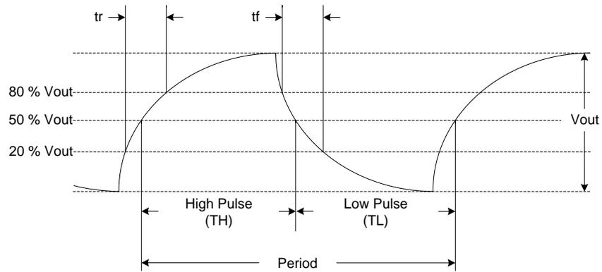
**Figure 16. Clipped Sinewave Waveform Diagram<sup>[11]</sup>**
