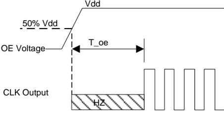
T\_oe: Time to re-enable the clock output
