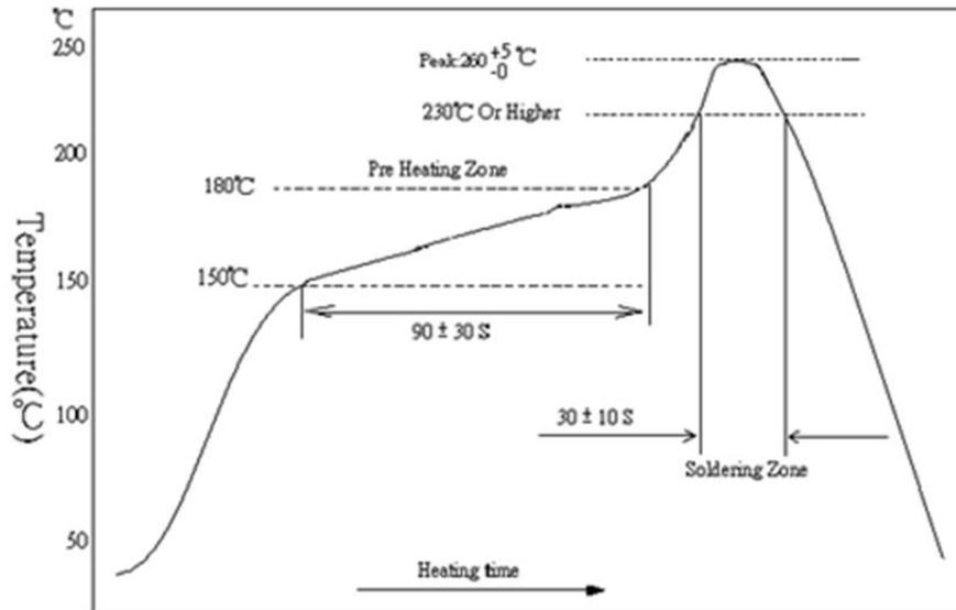
備註1: Recommended IR Reflow Soldering Profile 符合J-STD-020D;
