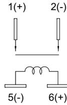
Load sides and coil terminals are with polarities (+) and (-).
