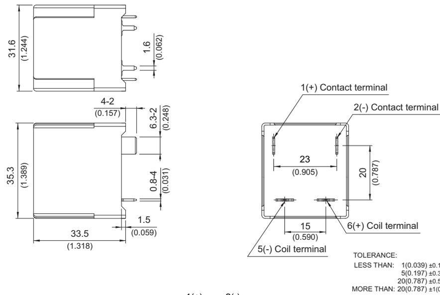
»» Wiring Diagram (Bottom view)
