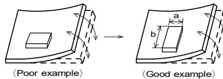
(2) Components location on PCB separation
