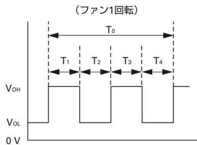
$T_{1\sim 4} \doteq (1/4) T_0$
