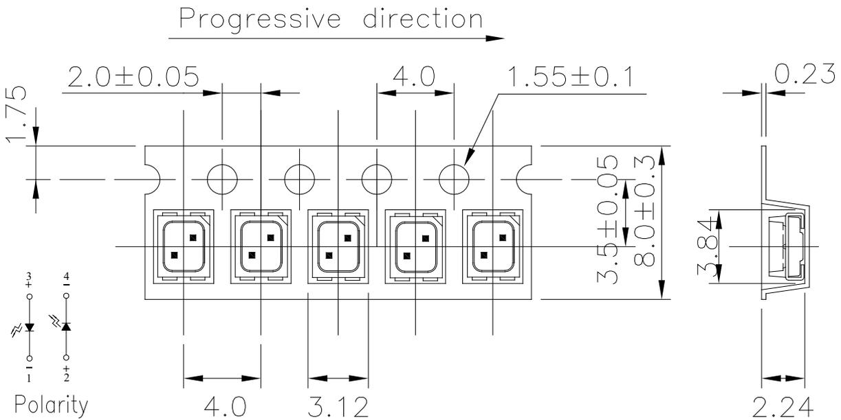
Note: Tolerances unless mentioned  $\pm 0.1$ mm. Unit = mm
