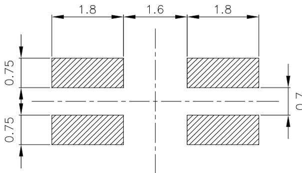
Note: Tolerances unless mentioned  $\pm 0.1\text{mm}$ . Unit = mm
